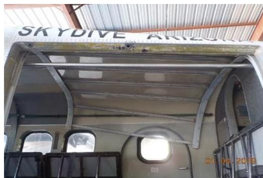
Door measurements are 127cm. high and 140cm. wide. A floater bar the length of the door is inside the plane. 84 cm. behind the door on the same level as the floor, is a videographer's step. Above and behind the door are videographer handles.
